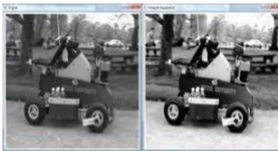
(a) Original Image (b) Enhanced image for Histogram Equalization
