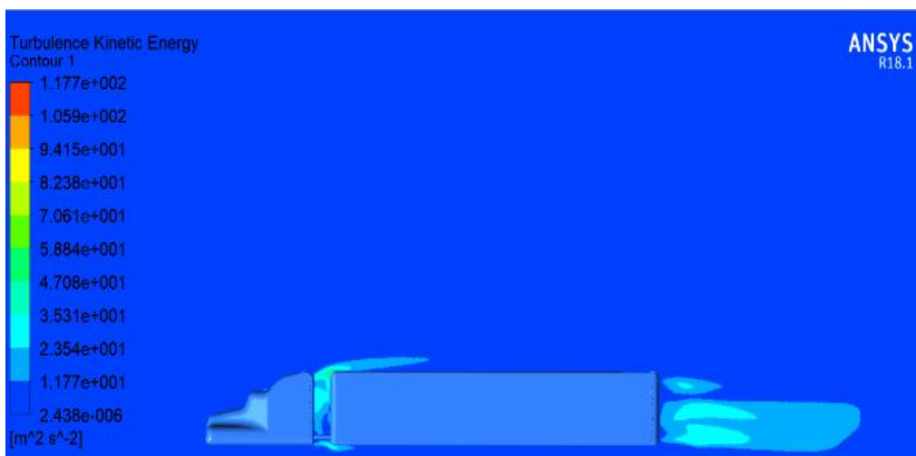
Fig.23 Turbulence kinetic energy contour (with Airtabs)
