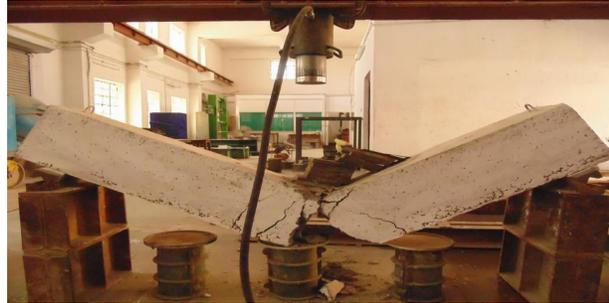
First Crack was observed at 50kN and beam failed in flexure at 120kN.
