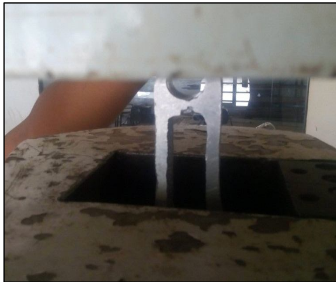
Fig: (9) After travelling lower jaw specimen is attached in to the upper jaw
