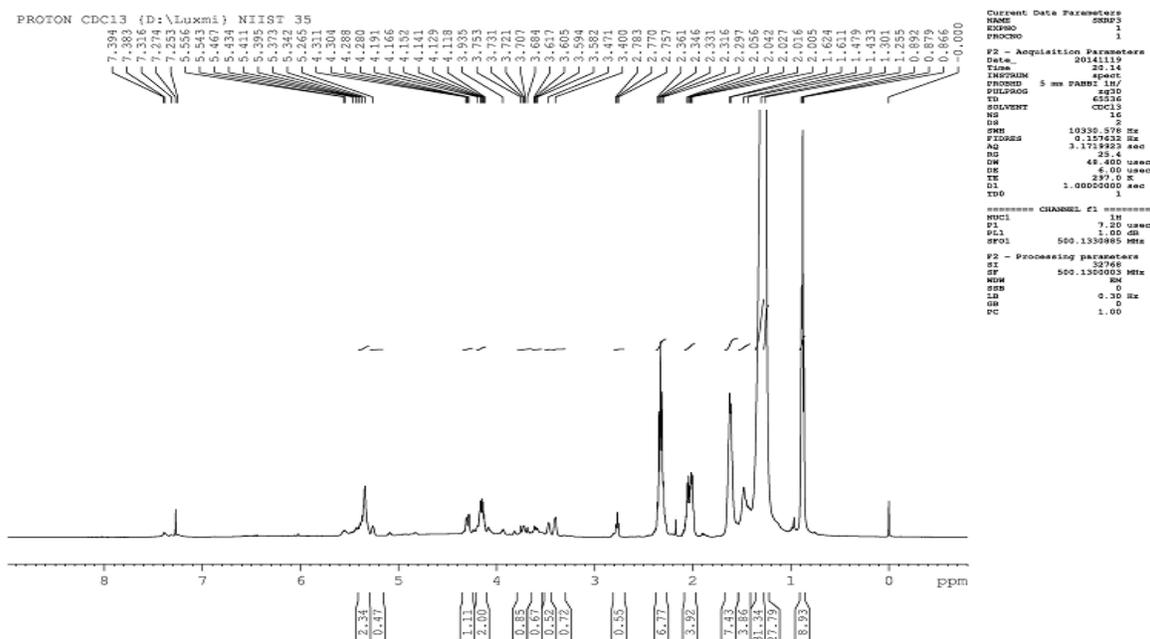
Fig 3 <sup>1</sup>H NMR spectra of epoxidised punnal oil
