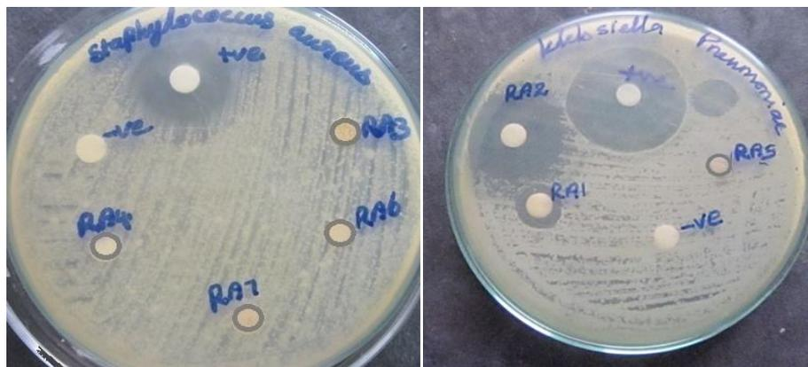
Fig 6 Culture plates of polyester and their composites with glass fibres using Staphylococcus aureus, Bacillus subtilis, Escherichia coli and Klebsiella pneumoniae.
