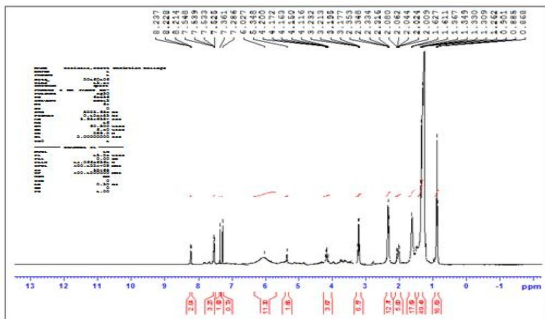
Fig 4 <sup>1</sup>H NMR spectra of anhydride based polyester resin
