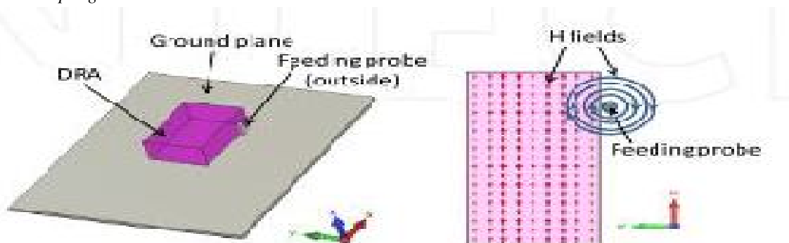
Fig.2 Coaxial probe coupling the H field
