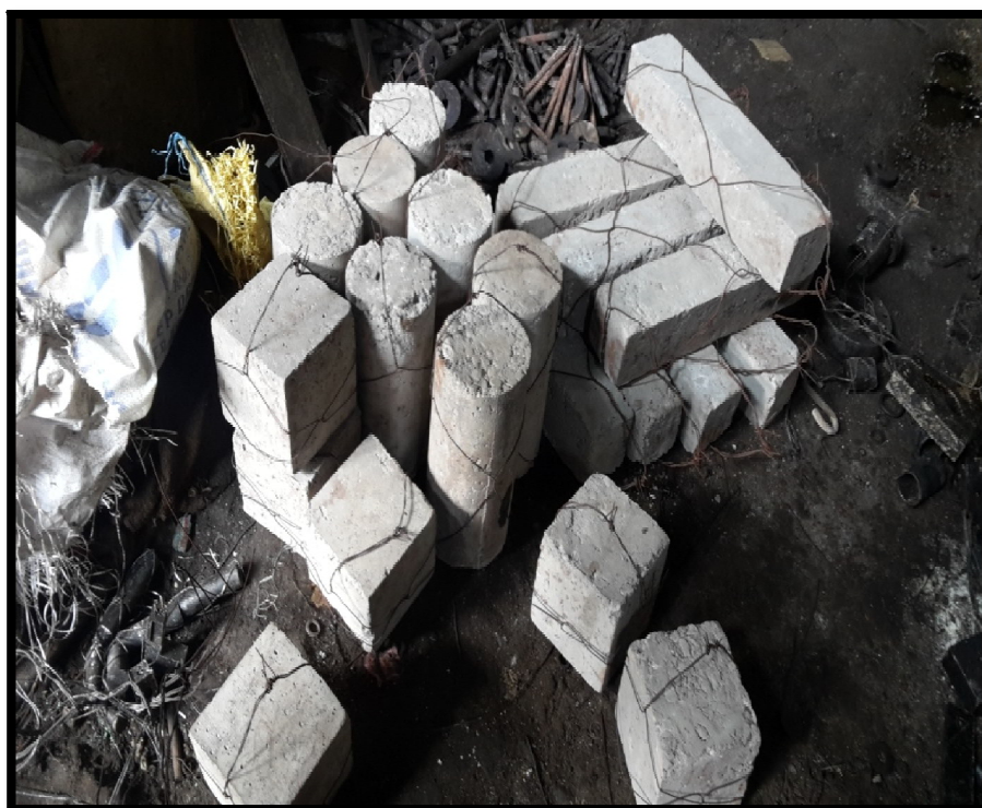
Figure 5. Concrete samples after fire test ( 400^{\circ}\text{C} and 800^{\circ}\text{C} )
