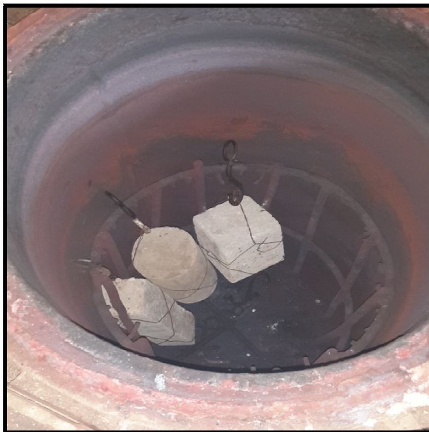
Figure 4. Concrete samples inside annealing furnace
