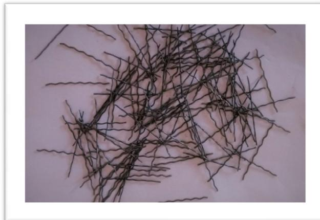
Fig 6 : Crimped steel Fibers
