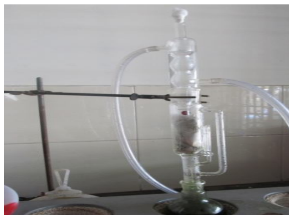
Fig.2. Solvent extraction by soxhlet apparatus
