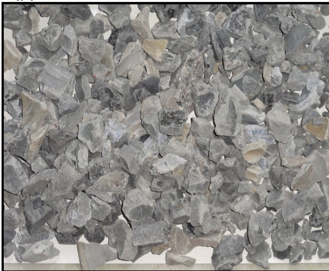
Fig.1 Waste Polymer Aggregates (WPA) derived from JaliGulla .
