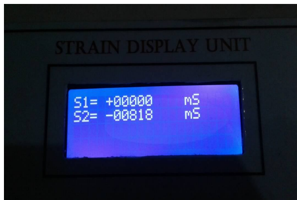
Fig. 24 Strain gage output 818 micro strains
