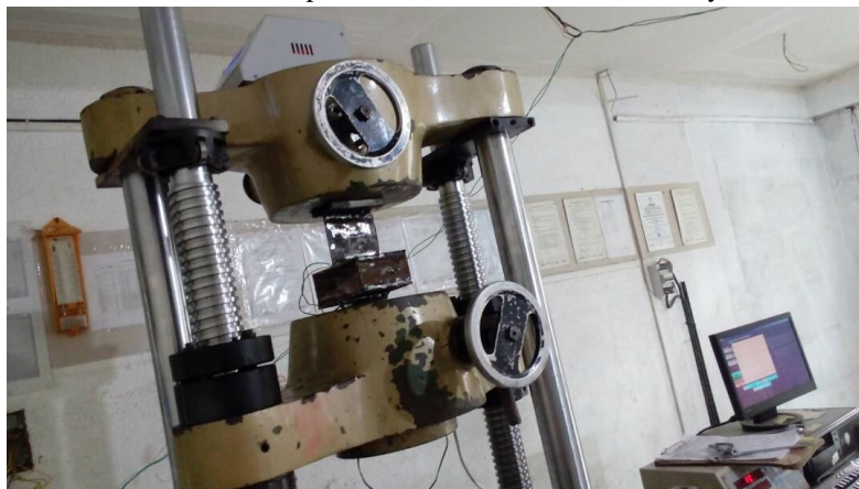
Fig. 21 Tensile Loading on T-Joint
