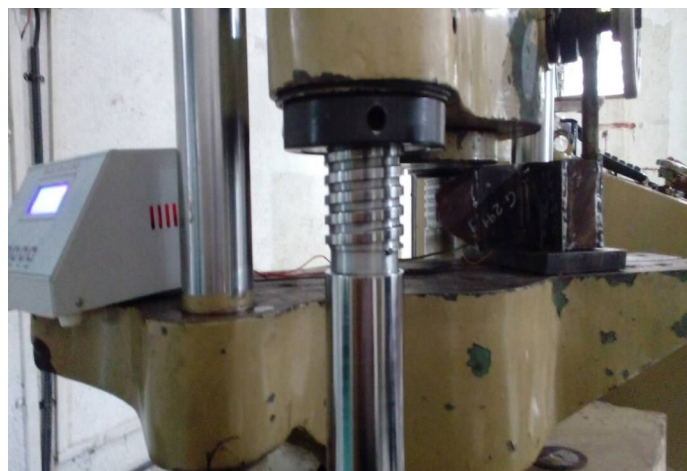
Fig. 23 Bending Loading on T-Joint
