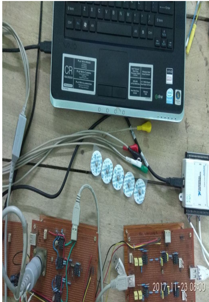
Fig. 6: Setup for Acquiring Speech Related EMG Signals
