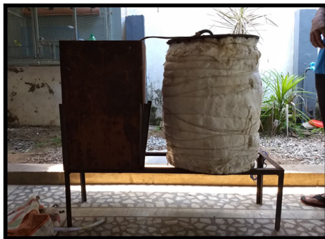
Fig.7 Waste plastic oil extraction set up
