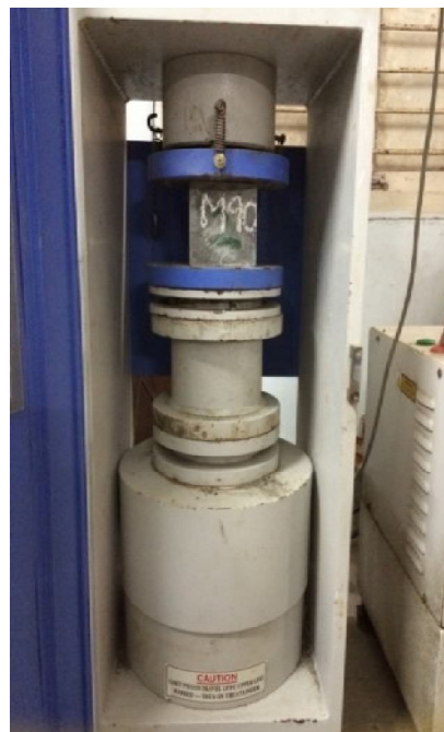
Fig. 3 Concrete cubes M 90 grade specimens in CTM
