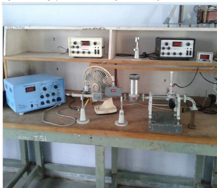
Fig.1 Experimental set up of x-band microwave bench set up
