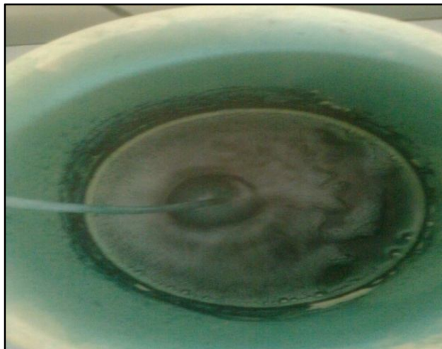
Fig-4 Aeration in SBR reactor.
