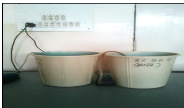
Fig-3: Experimental Set up of SBR
