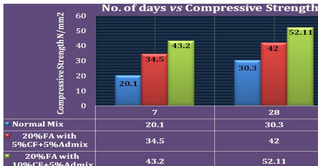
Fig 6 Compressive Strength of Concrete Cubes with: 5% & 10% of CF+5% Admixture with 20 % Fly Ash
