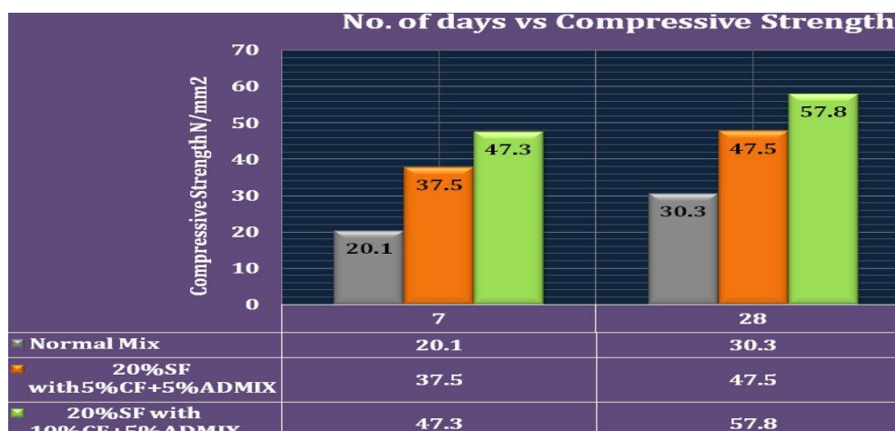
Fig. 4 Compressive Strength of Concrete Cubes with: 5% & 10 % of CF+5%Admixture with 20 % Silica Fume
