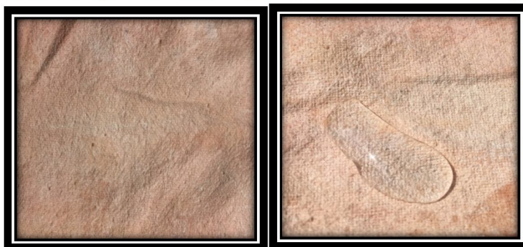
Fig 10(c) Cloth after Zinc sterate spray
