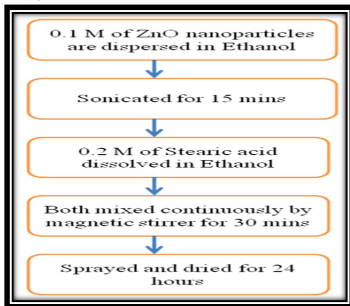
Fig. 2. Preparation of hydrophobic spray by ZnO nanoparticles
