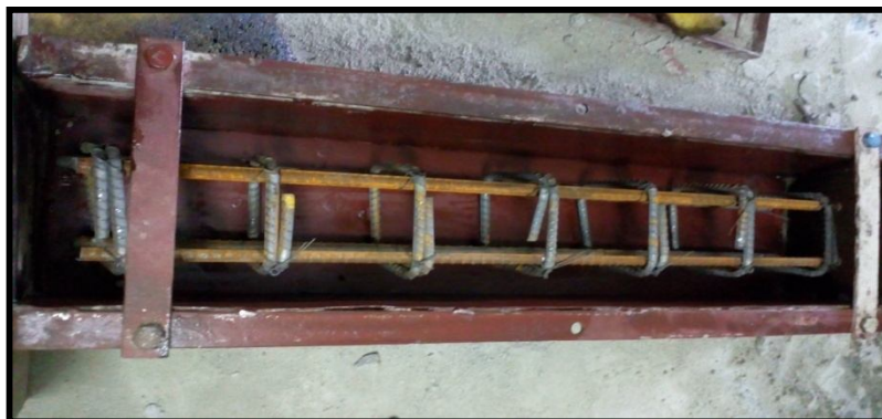
Fig.1 Reinforcement detail with mould
