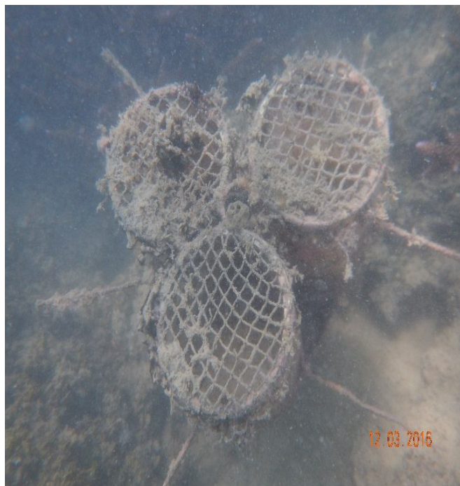
Figure 7 Exposed sediment trap for 80 days
