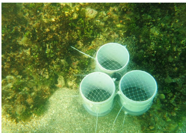
Figure 4 Erected sediment trap in the coral reef ecosys
