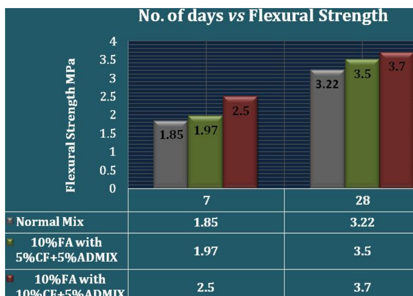
Fig 5 Flexural Strength of Concrete Beams with: 5% & 10 % of CF+5%Admixture with 10 % Fly Ash
