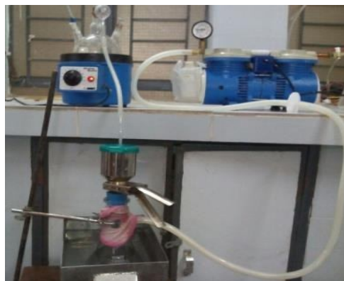
Figure 4- small pervaporation setup in lab
