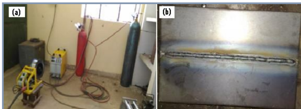
Fig. 1. (a). MIG welding setup, (b). Welded component.
