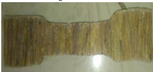
Fig 3: Test laminate of kenaf fiber
