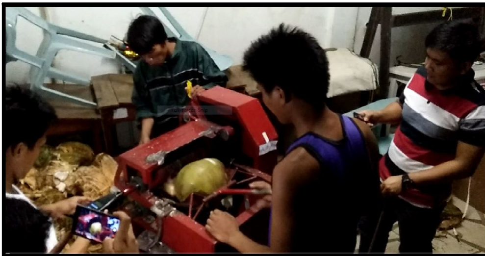
Figure 2. Actual dehusking operations of the machine during the final tests conducted by the researchers
