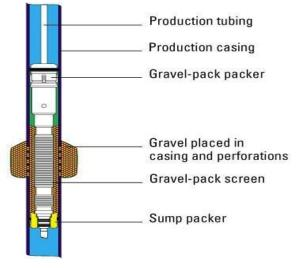
More entangled than establishing a well, rock pressing requires a slurry of properly estimated bits of coarse sand - or rock - to be drawn into the well between the opened liner of the packaging and the sides of the wellbore. The wire screens of the liner and the rock pack cooperate to sift through the sand that may have generally entered the wellstream with the hydrocarbons.
