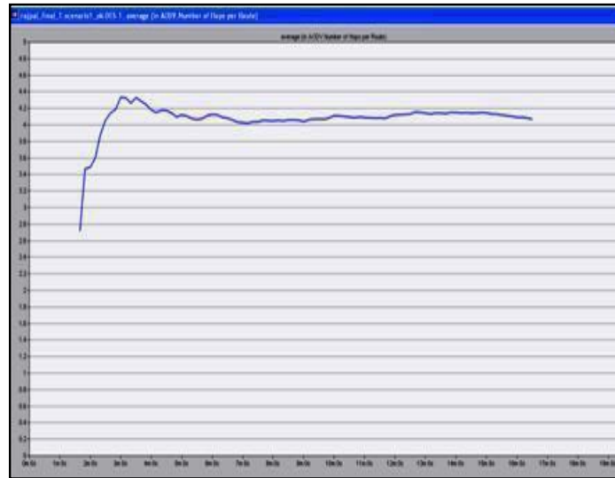
Figure 5.4 Average Hop count per route in scenario 1 without wormhole attack
