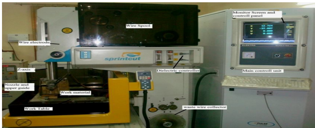
Fig.2.Experiment Setup of Sprint cut Wire EDM
