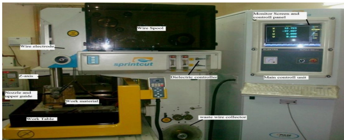
Fig.2.Experiment Setup of Sprint cut Wire EDM
