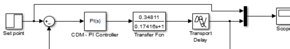
Fig 6: Simulink model for CDM - PI controller
