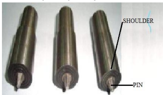
Fig 3.3 Tool used in Friction stir welding
