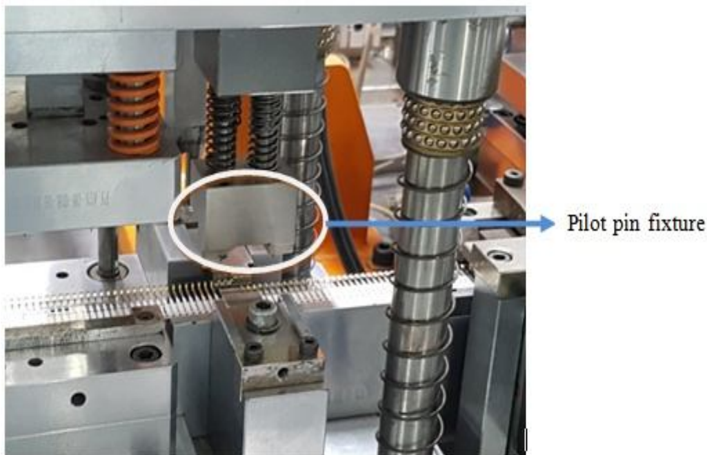
Fig. 10 Pilot pin implementation
