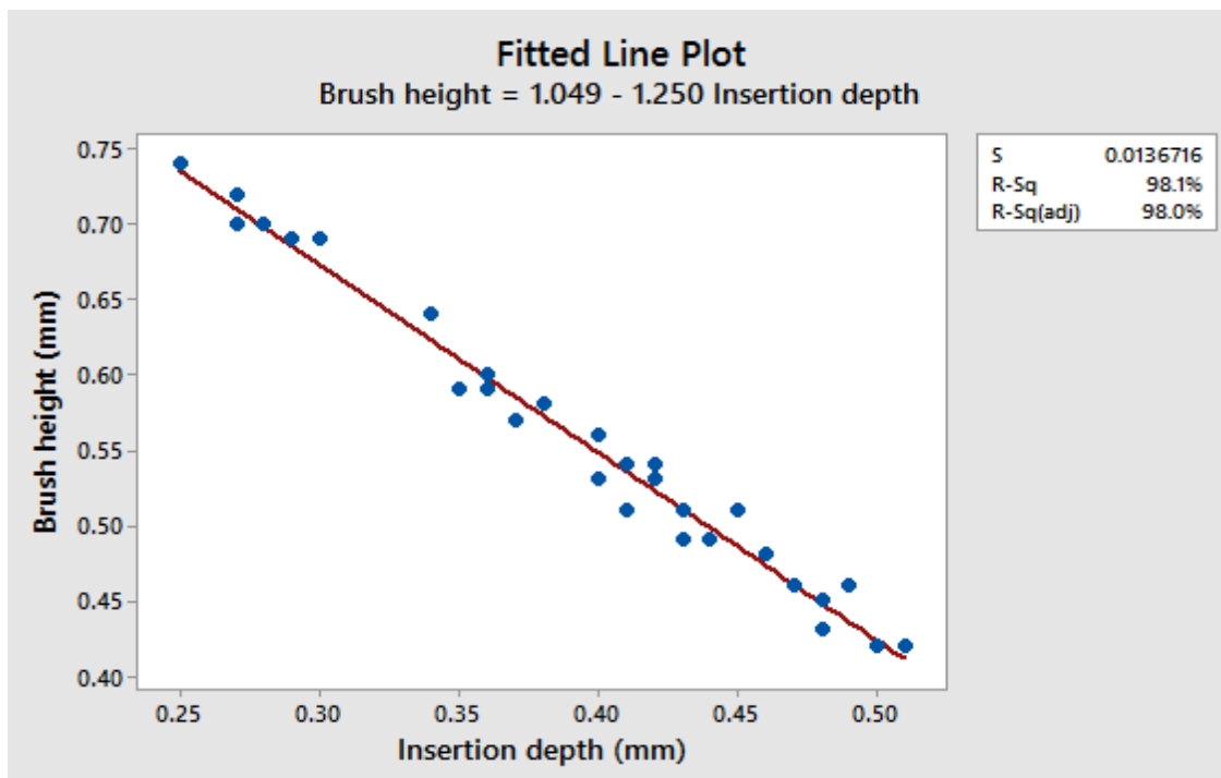
Fig. 8 Regression plot for insertion depth and brush height
