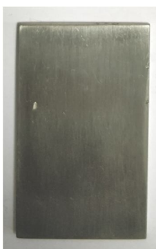
Figure#6 ASTM G48 Tested sample
