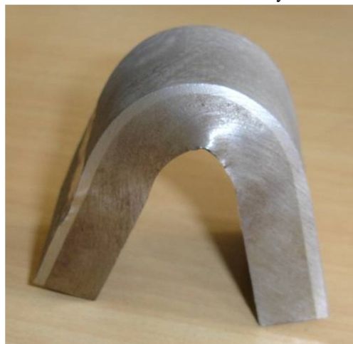
Figure #4 Bend Test Sample
