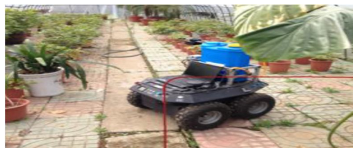
Fig. 3 Greenhouse turning tests of mobile robot
