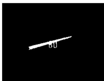
Fig. 10 Pointer Binary Images before Erosion
