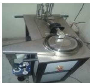
Figure 3: Pin-on-disc wear testing setup
