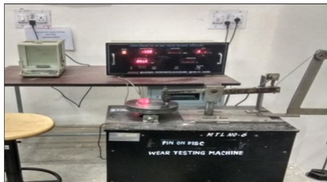
Fig: 2.5 Pin on Disc testing machine
