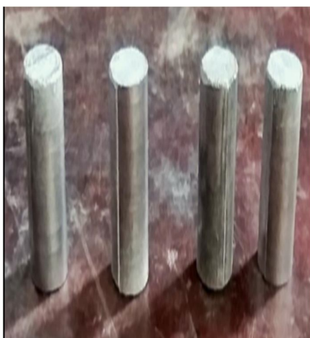
Fig.2.4 (a) Before sintering
