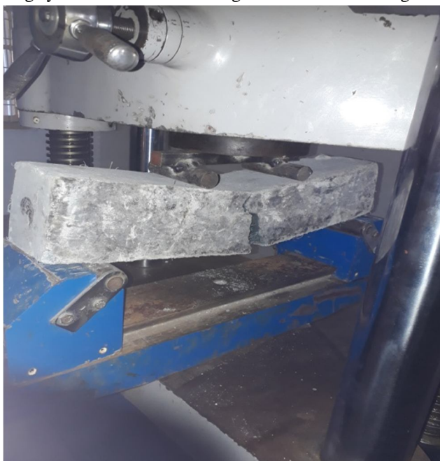
Fig. 12 Flexural strength Test
