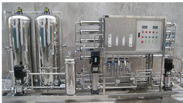
Fig 4. Commercial Reverse Osmosis Plant
