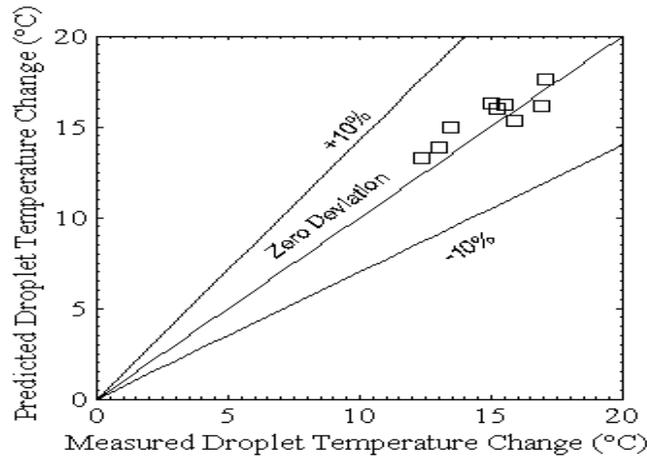
Fig. 2 Comparison of predicted and measured droplet temperature
