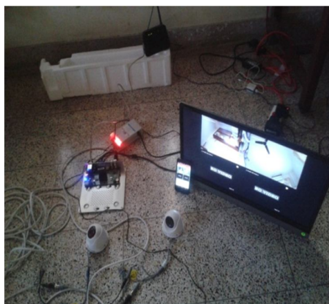
Fig. 3 IOT implemented CCTV with MDI Card
