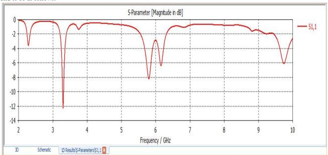
The dip near the ISM band (2.4GHz) is nearly -4dB while the next sudden dip occurs at around 3.4GHz with -12dB
