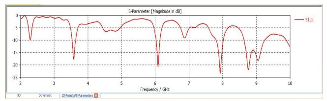
The modulation dips are found to be more frequent in the time domain starting with -10dB at the ISM band till nearly -25dB at 6.1GHz
