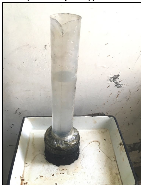
Fig. 5 Permeability test of Bituminous Samples
