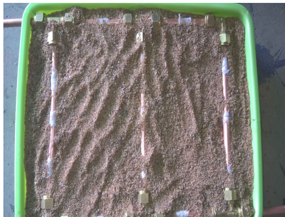
Figure 1: Set-Up of Copper pipes in Sand
