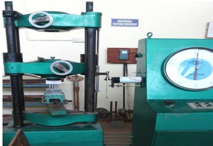
Fig 2: Compaction of powder by using UTM
