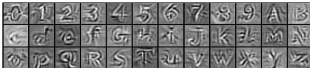
Fig.9 Filters learned from characters in natural images [19]. As can be seen, the learned filters can capture the shapes of the corresponding characters.
