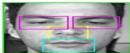
Figure 3: Face features (parts) identified by Voila-Jones algorithm (Boundary box) [1]
