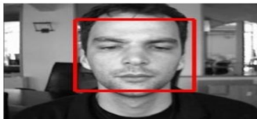
Figure 2: Face identified by Voila-Jones algorithm (Red boundary) [1]
