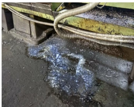
Fig. 1. Coolant wastage on lathe machine.
