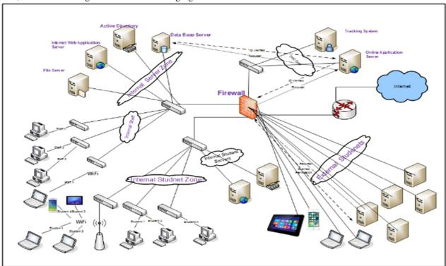
The information technology architecture shows the server confirmation, networks and various types of internal users and external students. The data is accessed and communications are through personal computers, laptops or mobile devices. In the suggested big data architecture, information management shows the data collection, storage, retrieval of data, analysis and output generation life
