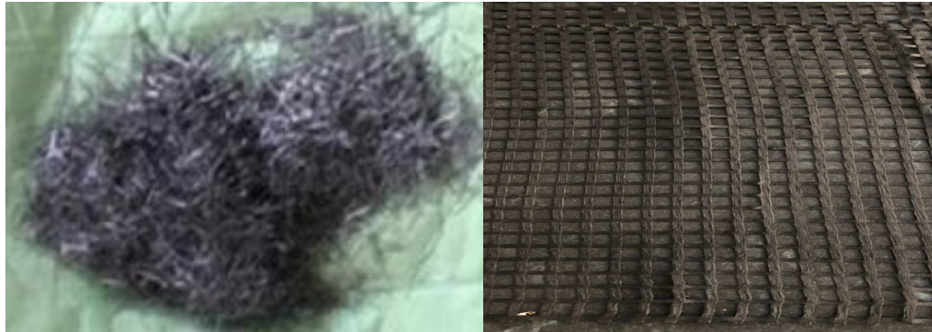
Fig. 1. (a) Hooked end steel fibre; (b) Bi-axial Geo- grid
