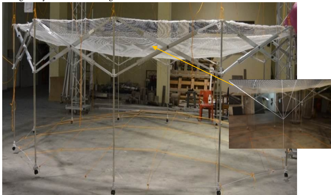
Fig. 4 Shape adjustment using ropes and strings
